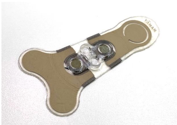
The stretchable FPC incorporating hydrogel used for the Stretch Fit Sheet
