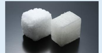
The NOXTITE acrylic elastomer has a number of well-balanced functions, including oil resistance, heat resistance, high strength, and resistance to permanent compression set. In addition to use as a material for oil seals and O-rings, it is used in devices that require heat resistance and oil resistance such as the surrounding surface of car engines.
