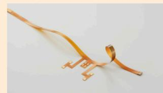
Single-sided FPCs (flexible printed circuits) have circuits on one side only. They are structured to best exhibit the thin and flexible characteristics of FPCs. They are durable against repetitive bending and can be used for space-saving wiring in moving areas. They are also suitable for multi-dimensional wiring in narrow gaps.
