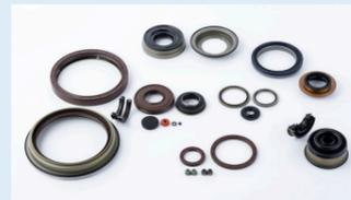
Oil seals are functional parts that seal oil. Composed of synthetic rubber, metal rings, and springs, they prevent oil from leaking through gaps in machine shafts and prevent dust and dirt from entering from the outside.
