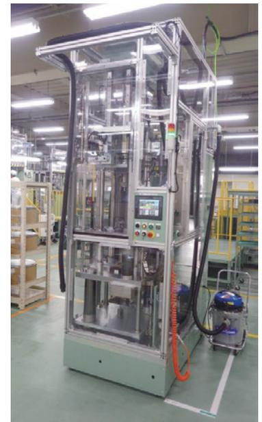
Energy efficient compacting press
