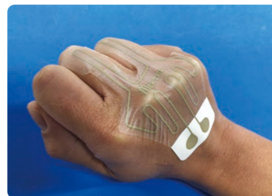
Stretchable FPC for a sensor to monitor biological signals
