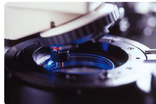
Oil membrane visualization equipment for oil seals used on rotating shafts
